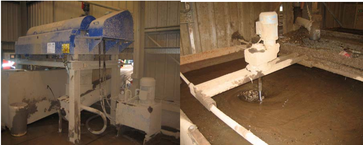
Example of a Hiller model DP45-422 centrifuge on mud / soil dewatering.
